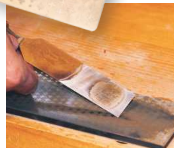
▲ The bench stone proved flat when tested with this pre-flattened chisel
